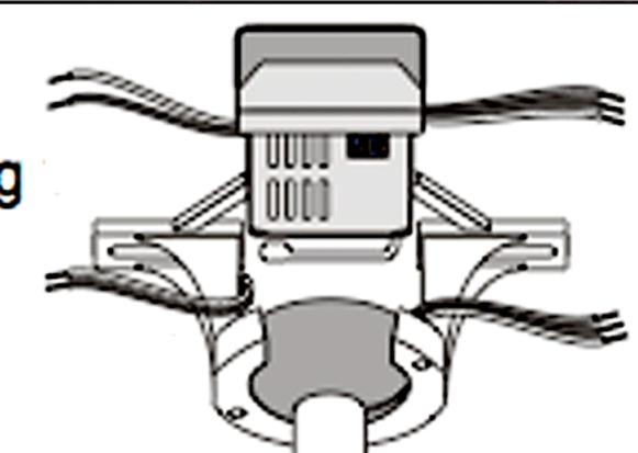
Now tuck the wires and wirenuts carefully into outlet box. Make sure the Green and White wires are tucked into one side of the box and the Black and Blue wires are tucked into the other side of the box. Make sure wirenuts remain tightly on connections.
