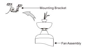
② Rotate fan so that the groove on the ball engages the ridge in the mounting bracket.
