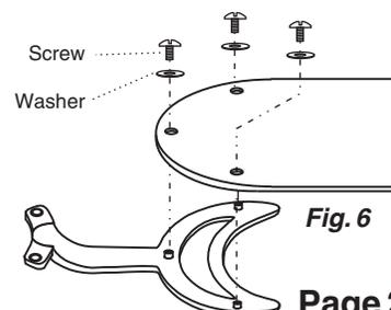
B. Snap together blade and blade iron. Note the side of the blade you want to show. Using the 3/16"-32x5/16" blade screws and 9/16" washers, three of each per blade, secure blade to blade iron. Repeat this procedure with the rest of the blades. You will have at least one screw and one washer left over, these are spares. Be sure all of the screws are tight. Fig. 6
