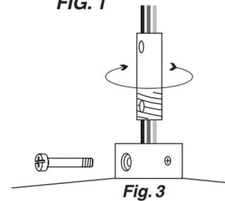
3. Insert the threaded pin and tighten it and the set screw.
