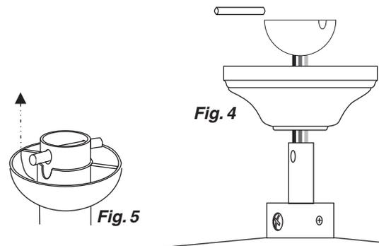
5. Raise the ball so that the pin is in the slot and tighten the set screw. See Fig.5
