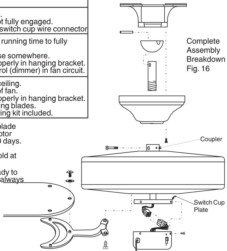
Complete Assembly Breakdown Fig. 16
