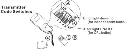
▲ Warning! CFL bulbs are not applicable to the remote with dimming function.
