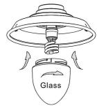
(2). Attach & rotate glass shade clockwisely to light kit pan.
