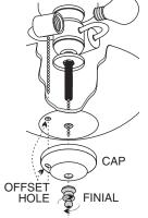
The offset hole is meant for the fan's pull chain.
